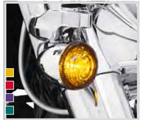
A. LED BULLET TURN SIGNAL INSERT KIT – AMBER (SHOWN WITH CLEAR LENS)
