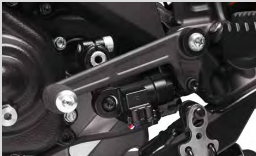
A. SCREAMIN' EAGLE QUICKSHIFTER FOR PAN AMERICA 1250 MODELS
