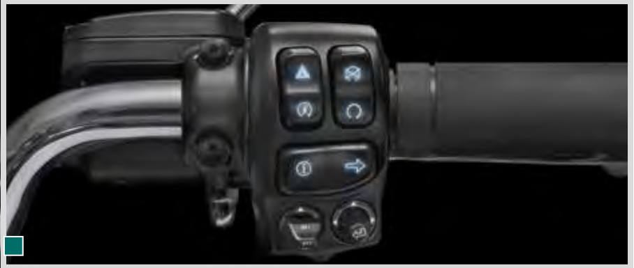
A. LIGHTED HAND CONTROL SWITCHES
