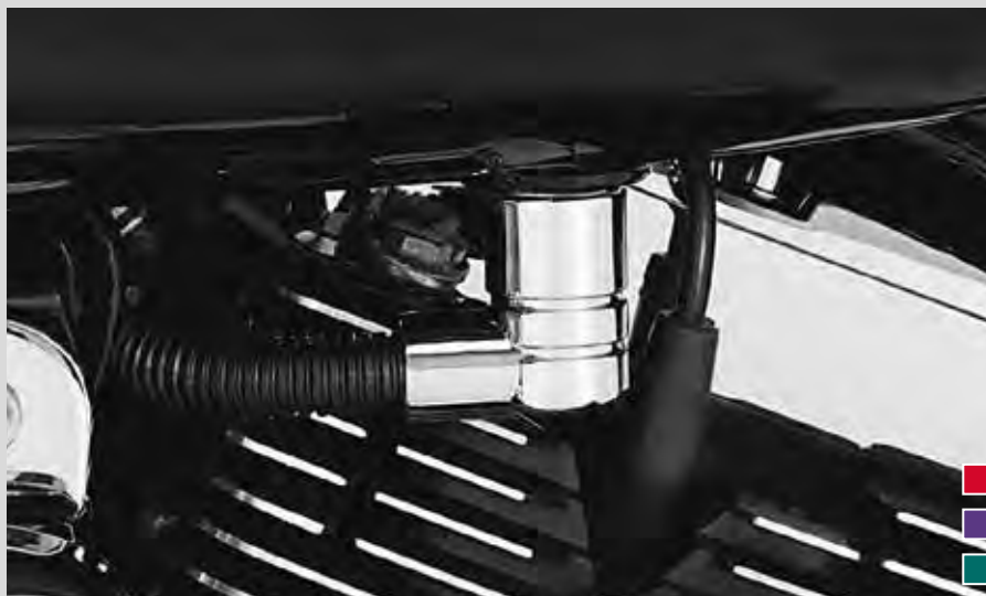
D. FUEL TANK FITTING COVER
