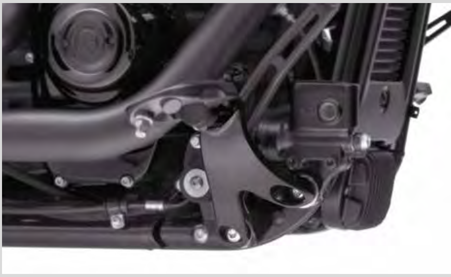
C. ORIGINAL EQUIPMENT FOOTBOARD-TO-FOOTPEG CONVERSION KIT
